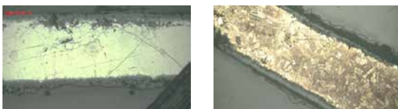
Fig. 5. The microstructure of metal vessel No. 2 (2-251TA) shows numerous slip lines indicative of hammering, and intergranular corrosion is visible (magnification \times 200 ). Source: Author's archive.
