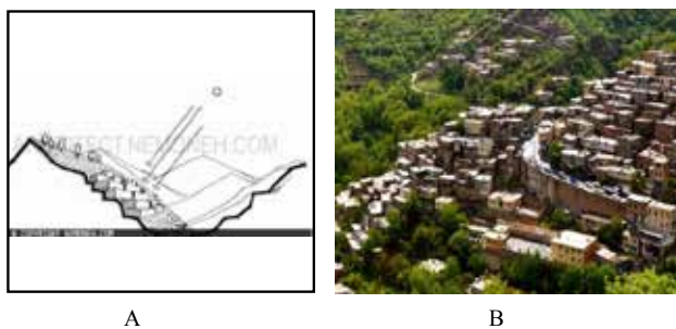
Fig. 2. A: House buildings on steep mountainous slope Source: www.architect.nemoneh.com. B: Nowdeshah city; the roof of every house is a yard for the upper house. Source: author's Archive.
