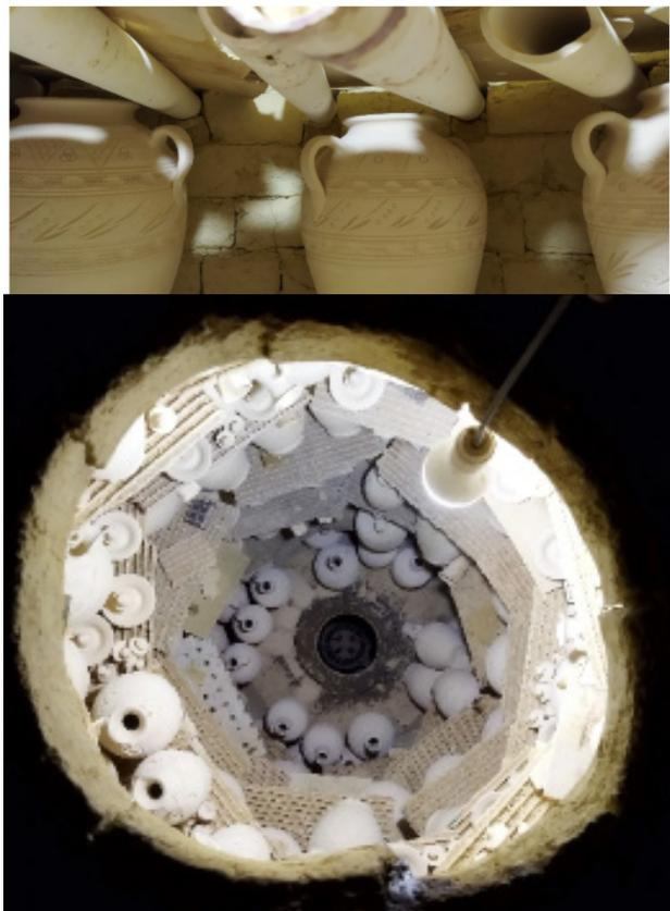
Fig. 8. Traditional kiln. The ceramic tubes that are placed inside the kiln body to hold the ceramic plates. Source: Authors.
